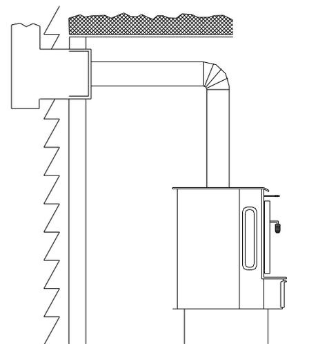
FIGURE 9 - INSTALLATION INTO A FACTORY BUILT CHIMNEY
