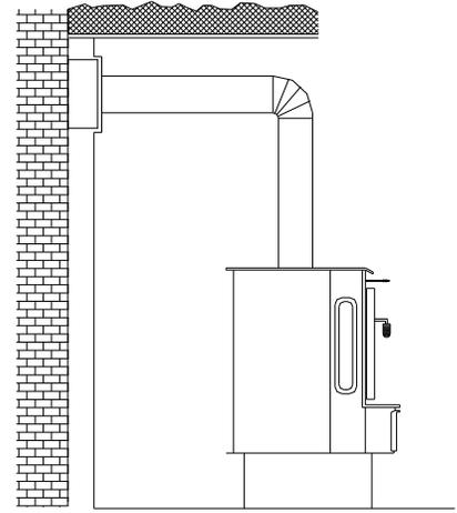
FIGURE 8 - INSTALLATION INTO A MASONRY FLUE
