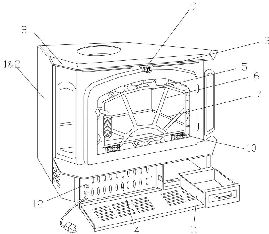
1. Quality steel construction - assures you of years of dependable service. The firebox is constructed of 4 gauge plated steel that is completely welded for safe, durable installation.
