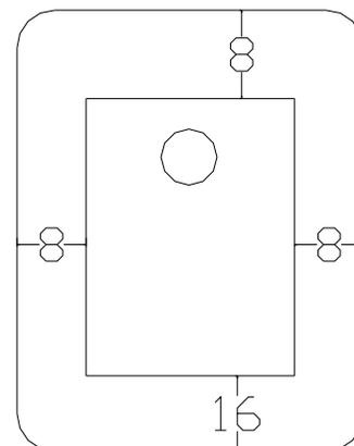
FIGURE 3 - CLEARANCE TO COMBUSTIBLES
