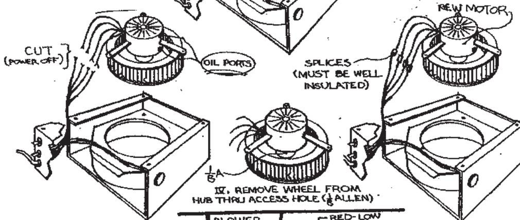
IX. REMOVE WHEEL FROM HUB THRU ACCESS HOLE (1/8 ALLEN)
