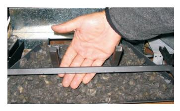
Step 4: Once the wool is in place, check the gap between the grate bar and the wool. It should be about the thickness of your hand. (Approximately 3/4")\_
