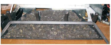
Step 3: Place wool in a single layer from the first ledge continuing to the top of the burner.
